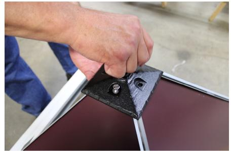
Slide the 4th Roof Panel on from right to left, tucking the tab under the panel on the right side as it is slid into place. Use a screwdriver or small putty knife to start roof on extrusion and also to keep it from scratching the roof panel on the right. (See Picture 11.)
