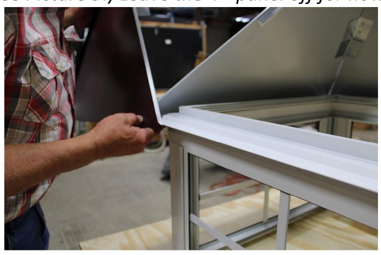
Align roof panel edge support tabs on corners under each of the panels.
