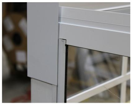
Place the Roof Rails on the top of the lited side assembly, aligning them in between the corner trim and the window extrusion. Align the corners and attach with two (2) #8 PPH screws in all four corners. Use care not to overtighten screws. (See Picture 5.)
