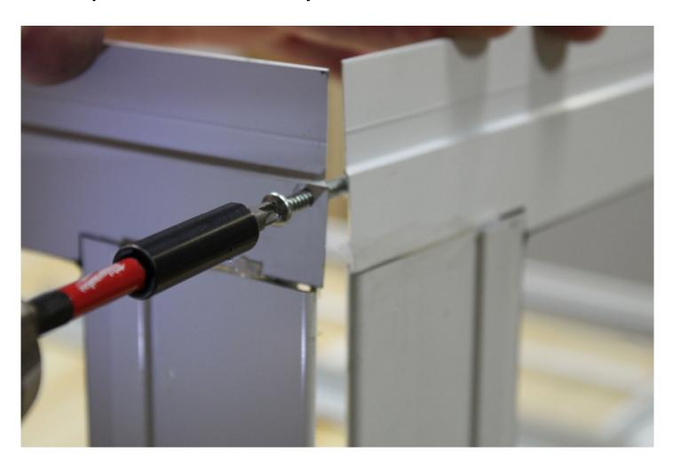
Place the 4<sup>th</sup> Side Panel in between panels #1 and #3 as shown. Assure alignment, and drive the remaining six (6) screws similar to the other joints. (See Picture 4.) Tighten all screws using care not to overtighten.
