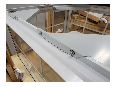
Four (4) #10 x 1" self-drillers with washers are installed in each pre-formed corner gusset. Completed four-sided lited side unit with gussets installed shown. (3' & 4' cupolas only).
